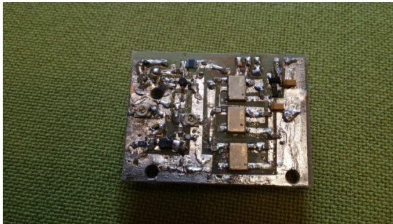
Foil &amp; component side with the 3 Epson chips
