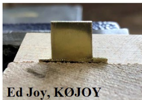
Filing Fixture Used to Achieve Final Dipole Shape
