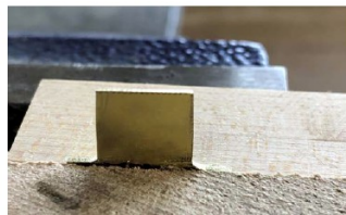
Filing Fixture Used to Achieve Final Dipole Shape
