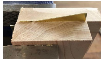
Filing Fixture Used to Achieve Final Dipole Shape
