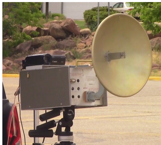
AB0MY's 10GHz, DVB-T transverter with 12" dish antenna and waveguide feed
