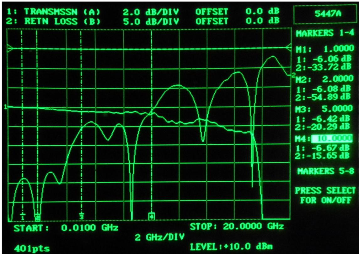
S21 & S11 of Amazon, 6dB, SMA attenuator. Sweep from 10MHz to 20GHz. S21 plot at 2dB/div. is top curve #1 starting from the left side. S11 plot at 5dB/div. is the bottom curve #2 starting from the left side. Markers show measured values at 1, 2, 5 & 10 GHz. Measured on Wiltron model 5447A Network Analyzer.
