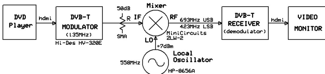
Fig. 1 Test set for mixer/LO tests of DVB-T
