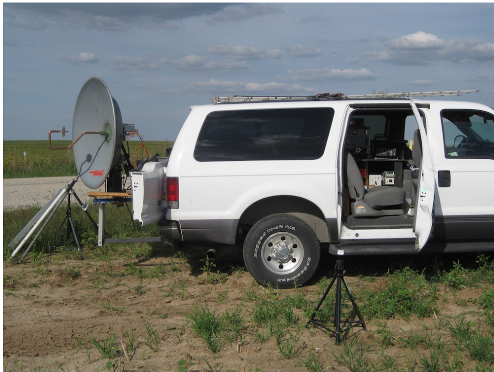
Phil, W6HCC's 10 GHz rover setup. 4 ft. dish with waveguide feed and 8 watts of RF power from a solid-state amplifier.
