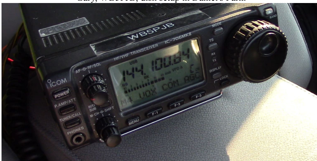
Gary' 2 meter, SSB rig listening to Bill, K0RZ's 10,368.100 MHz SSB signal, peaking at S9 +40dB !!!
