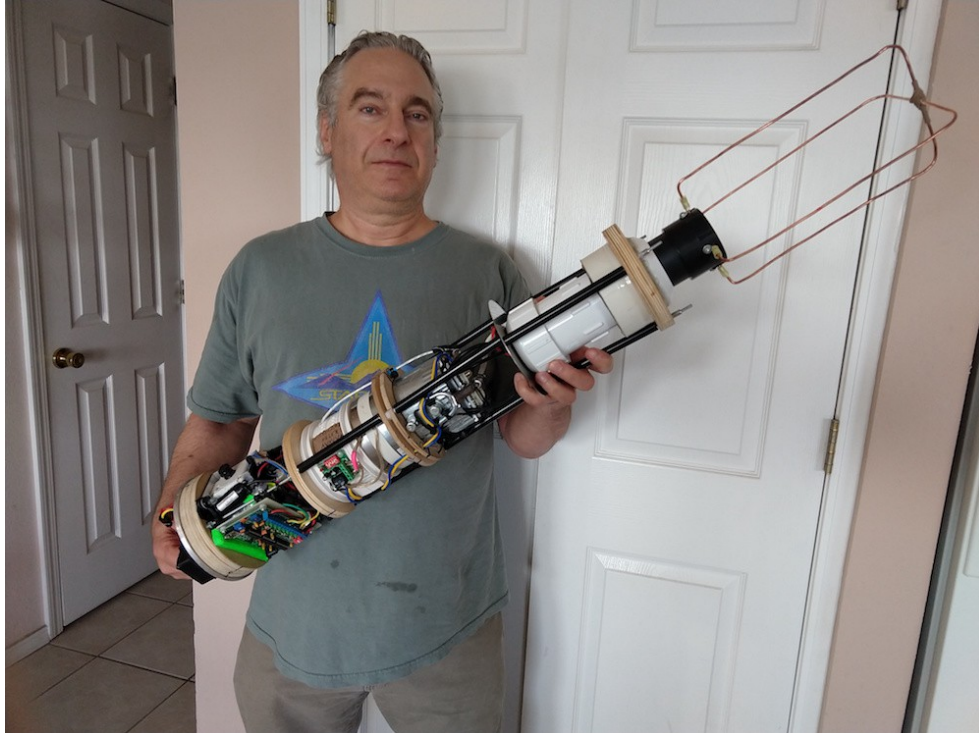
Ken, KD5EH, holding the transmitter package with the rib-cage antenna.
