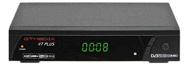
We have recently discovered a new, low cost, combo DVB-S & DVB-T set-top box receiver which will also tune the amateur 70cm & 33cm bands for DVB-T. It is the GT Media V7+. It is available in stock in the USA from Amazon Prime and sells for \$42.
