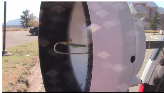
Don's SSB / DVB-T, 9cm transverter & dish antenna with log-periodic feed
