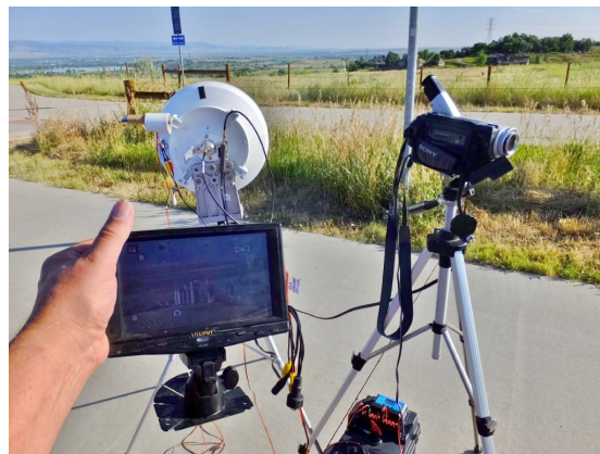
Chris, K0CJG, setting up his microwave gear (left) on the US-36, Boulder Overlook & receiving a signal from Don, N0YE, at Rabbit mountain (right) 19 miles to the north.
