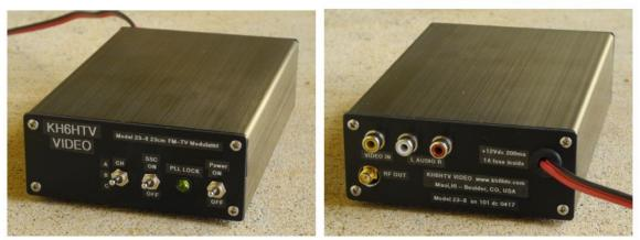
The model 23-8 is a 23cm, analog (NTSC or PAL), FM-TV modulator. With 50mW (+17dBm) rf output it is ideal to drive high power amplifiers for an FM-TV transmitter. Frequency synthesized on 3 channels. For more details: www.kh6htv.com
