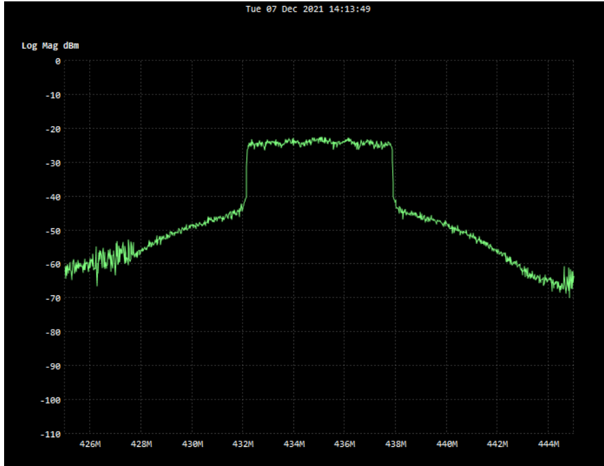
Fig. 6 435MHz, 6 MHz BW, 0dBm DTV signal measured directly on the TinySA, using the HIGH, UHF input.
