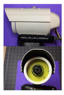
The HiDes DC-105 is a Full HD DTV (1920x1080x30P) Camera that supports transmission in the frequency range of 70 to 1450 MHZ. The DC-105 is available in 3 iterations; one with a cubic housing and a small stand, a bare bones model without a case and a third version with bullet housing and stand. The model I purchased was installed in bullet security camera style housing. This model and its use in Amateur TV is what this series of articles are about.
