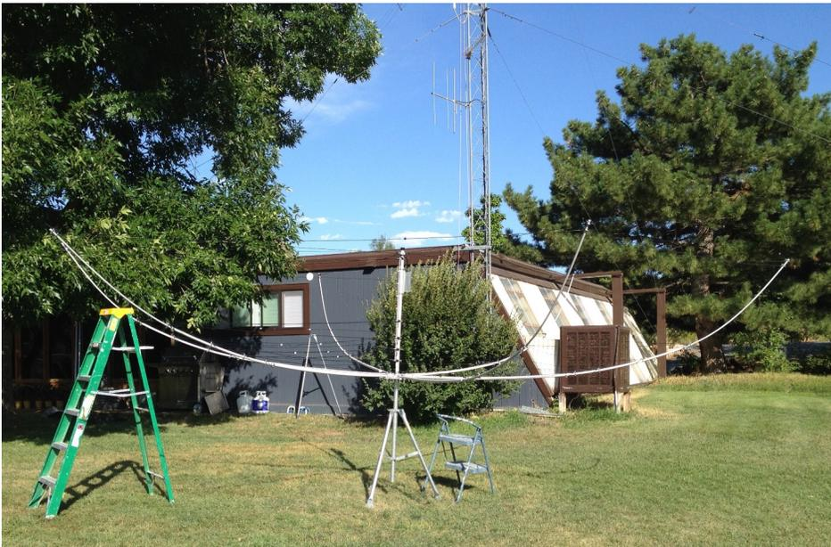
Finished Hex Beam Antenna --- assembled at ground level. Mounted on 3 ft. pipe in tripod. Worked Hawaii on 17m as is !!!
