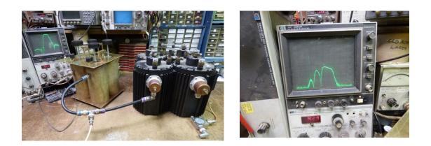
**DUPLEXER for Omaha** -- John, WB0CMC, writes us ---"Initial testing for an in band ATV duplexer. Photo on left is ANT to RX, 434 passband Photo on right is pass through RX-TX. Next stage is put a TX into a dummy and check RX RFI/desense. Looks promising, so far. Marker on 003 is 421.25.
