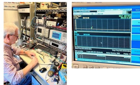
Tom at the helm conducting the Noise This is the Agilent EXA Signal Analyzer Figure and Gain Measurements on the VHF that Tom used for this test measurement. Designs preamp for 70cm
