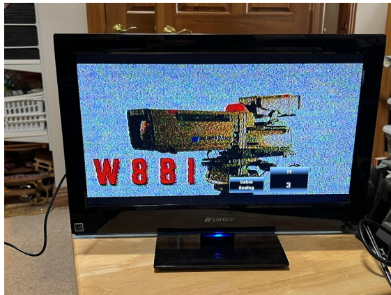
Left Photo: SANSUI Model SLED1980D Receiving a “P3” A5 Video from the W8BI ATV Repeater site
