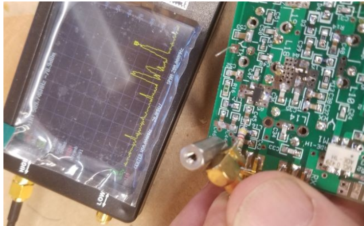
Fig. 1 Probing RF circuit with Spectrum Analyzer thru isolating resistor probe.
