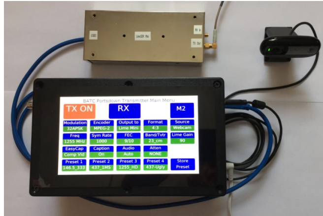
The BATC Portsdown Transmitter and LimeSDR
