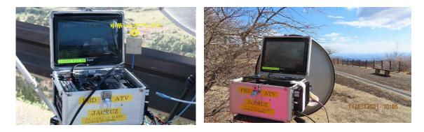
Here is a picture of my 5.7GHz Full HD-ATV transceiver. With a 10.2 inch monitor, you can send, receive, record, playback and send back his Full-HD footage on his ISDB-T. It can be changed with one switch. Full HD-ATV communication of 110km was successful even with a small patch antenna directly attached to the transceiver in the photo.
