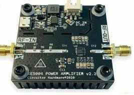
SE5004. The pc board is mounted directly to a heat sink. The connectors are SMAs. The photo shows a pi attenuator on the rf input (R9,10&11), but the it is not present on the actual amplifier. R9 is simply a 0  $\Omega$  jumper.
