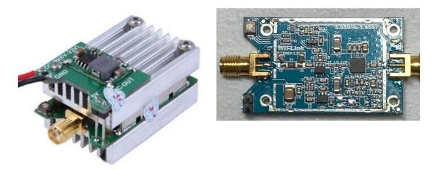
**SE5004 - Amp #2:** This is the amplifier currently marketed on the internet as the "After-Burner" for drone 1/2 Watt, FM-TV transmitters. They claim 2 Watts output. It currently typically sells for \$25-30 on E-Bay.
