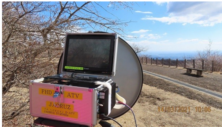
Figure 1. 5.7 GHz FHD-ATV operation in Nagano prefecture, Japan (Once the antenna and power supply are connected, Full-HD video transmission, reception, and recording are possible immediately.)
