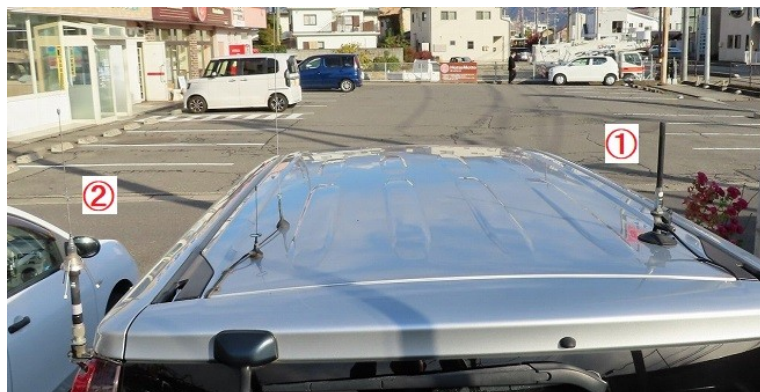
Figure 7. Mobile antennas attached to the vehicle roof. (1) is a 3-stage collinear antenna for 5.7 GHz (2) is an antenna for 1.2 GHz
