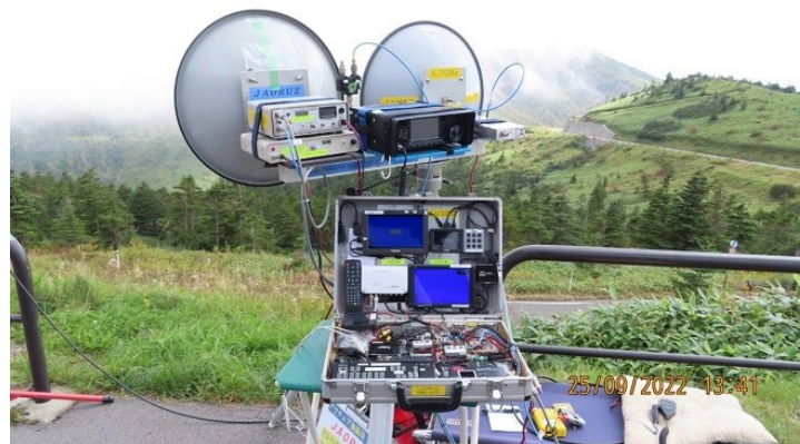
Figure 2. 10 GHz transmitter/receiver (AV, monitor, IF, and so on. are separately incorporated in the trunk)
