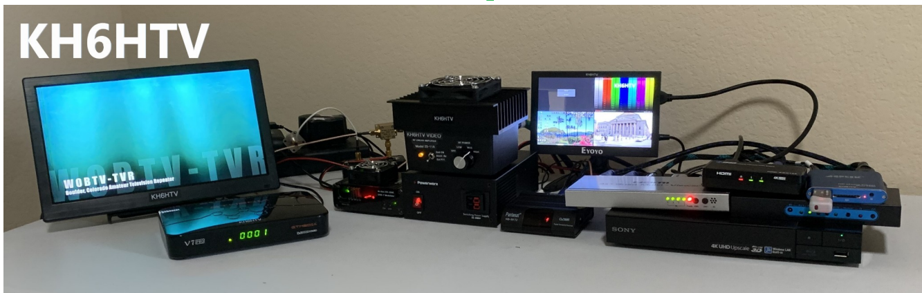
The KH6HTV DATV Video Studio, 70cm Receivers & 23cm Transmitter
