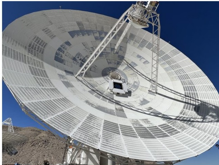
Capable of receiving both radio frequency and optical signals, the DSN's hybrid antenna has tracked and decoded the downlink laser from DSOC, aboard NASA's Psyche mission. Read More
