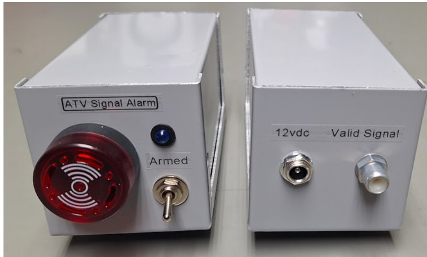
Completed Valid Signal Alarm
