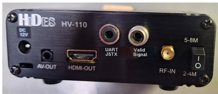
Rear panel Valid Signal* is connected to a standard RCA jack. The other jack is a 1/8 th inch mono connected to J5, the UART debug port. *Credit to KH6ATV for circuit used for Rptr PTT line.
