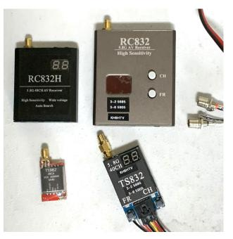
Basic RF specs. are similar, except the new units are programmed for 48 channels vs. 40 channels. But the size is dramatically smaller as shown in this comparison photo. The transmitter pc board is only 0.8" x 1.3" in size. Biggest item on it is the RP-SMA connector
