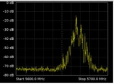
*IC-905 FM-TV* Comparison of FM-TV spectrums: center freq. = 5.650 GHz, span = 100MHz, 10dB/div & 10MHz/div
