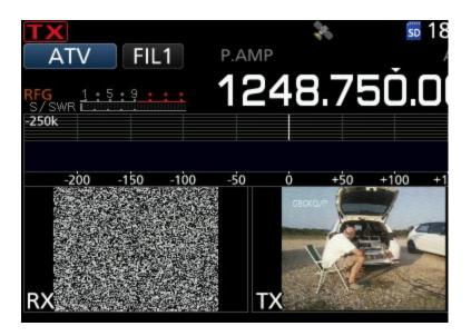
The transmitted picture can be shown alongside the received picture on the touchscreen; either picture can be enlarged to full-screen simply by touching it. Sadly, the frequency tuning control is disabled when full-screen is selected. An external monitor can be connected to display (or record) the received pictures, and stills can be saved to an SD card inserted into the controller.
