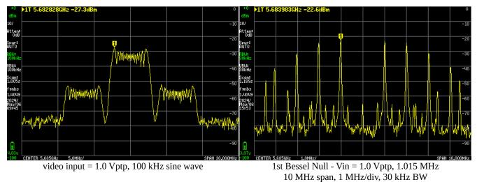
Based upon the measurement of the 1st Bessel function null at about 1 MHz modulation frequency, I estimate the transmitter's deviation to be about 2.5 MHz. Based upon the "live" video measurement, it appears that the practical -20 dB occupied band-width is of the order of 7 MHz. When one includes the 6.5 MHz SSC sidebands, the occupied band-width is considerably wider at about 15 MHz.
