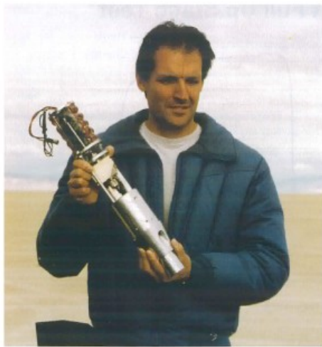
Mike Henkoski holds up the video package he put together on such short notice. The oval hole in the boat tail is the port through which the camera viewed the ground. At right, he is holding the fully assembled dart after a test fit of all components in the field.
