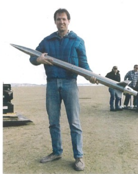
Mike Henkoski holds up the video package he put together on such short notice. The oval hole in the boat tail is the port through which the camera viewed the ground. At right, he is holding the fully assembled dart after a test fit of all components in the field.
