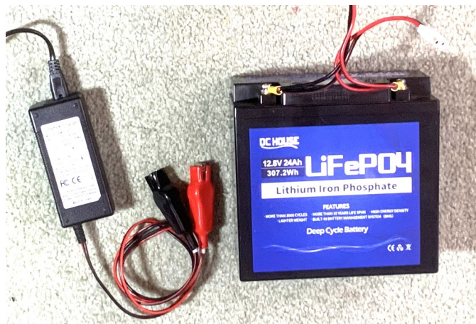
12Vdc high capacity Battery & Smart Charger
