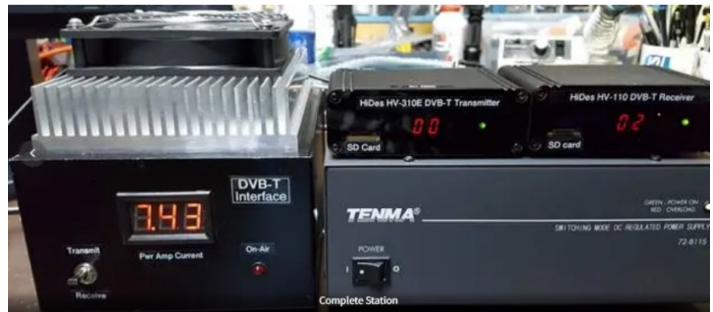
Typical Digital ATV Station. Just add a TV, camera and antenna.
