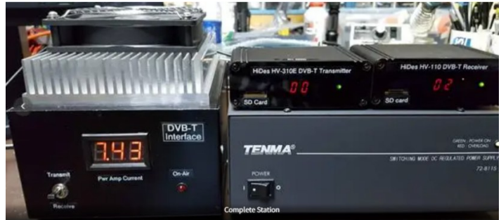
Typical Digital ATV Station. Just add a TV, camera and antenna.
