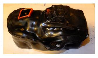
"I walked out to my garage/lab and opened the door and was engulfed in a cloud of dense black smoke. I had a meltdown of a lithium polymer battery pack for an electric drill (unknown brand Chinese import, purchased ~2 years ago). Apparently, the charge management circuit failed and charger
