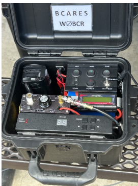
BCARES, 70cm, 3W, DVB-T Transmitter
