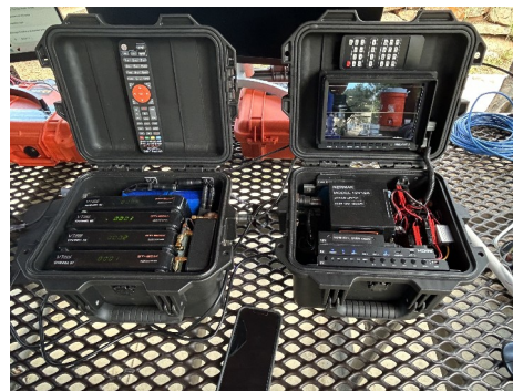
DVB-T, 70cm, Quad Receiver (left) & HDMI quad viewer
